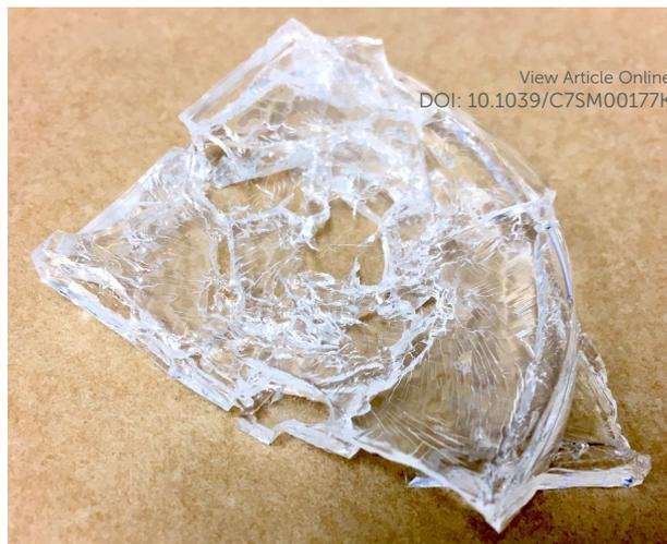
FIG. 18: The 1:30 PDMS elastomer after swelling in hexane and drying the sample.
